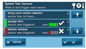
During the walk test, the Control Panel displays the signal strength of the RF transmissions received from each of the sensors. This helps to identify any sensors with a weak signal at the Control Panel.
