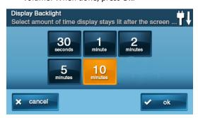
To view the 2nd Toolbox Screen, press  $\rightarrow$ . To set the display lighting timeout, press **Back Light Timeout**. Choose the length of time that the display will remain lit after it is idle. When done, press **Ok**.
