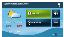
The Home Screen shows the system status with icons to indicate system conditions. It also displays the time and date. System information scrolls along the top of the display. The Home Screen displays the Security and Services buttons and the Silent Control and Display Off buttons. Pressing the Control Panel's A button displays the Home Screen.
