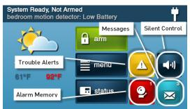
The Security Screen displays 3 buttons for Arm, Menu, and Status. The Silent Control button and the time and date are also displayed. If messages, alarms, or trouble alerts are pending, it displays buttons indicating the number of pending messages or issues.
