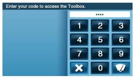
The **Installer Toolbox** button enables accesses to the Installer Toolbox used to program the system. Before access to the Installer Toolbox is allowed, installers must enter their installer code in the Installer Code Entry Screen. The installer code does not disarm the system.
