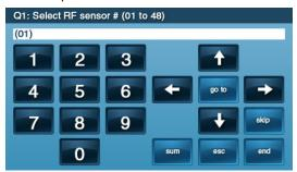
The **Go To** button is used to jump directly to a programming question. Pressing Go To prompts the installer for the two-digit question number to jump to. The Go To button changes to Cancel while waiting for a question number. Press Cancel to back out.
