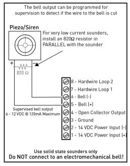
WARNING: DO NOT connect an electromechanical bell to these terminals. Damage to the output will occur.
