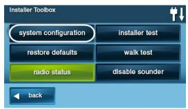
The Installer Toolbox Screen displays system setup and testing buttons. Main programming is accessed using the **System Configuration** button. The other buttons support system tests and resetting the Control Panel to its programming default values.
