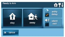
The Arming Screen is used to arm the security portion of the system. It displays the system status and arming buttons for Stay and Away. Option check boxes for Entry Delay and Silent Exit are displayed. To arm the system without an entry delay, un-check the Entry Delay check box. To arm silently without sounding the Exit Delay beeps, check the Silent Exit check box. Stay Mode arming always has a silent exit.
