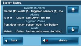
The Status Screen lists system status and any alerts. The date and time of alerts are listed in the displayed log. One option button for Silence is displayed; it temporarily stops the announcement of the system status during the status display.
