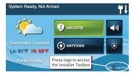
2 Press the logo at the lower right corner of the screen. (The **Installer Toolbox** can also be accessed via the third screen of the System Toolbox, but this takes longer.)
