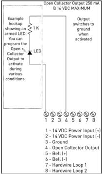
This output only functions while the Control Panel is receiving power from the wall power supply.
